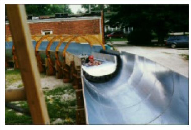
Figure 1. The Aeromobile 17 moving frictionlessly at speed with thrust from a slight tilt of the Gimbal Fan on the curve of the Aeroduct ROW. It is shown slightly banked by centrifugation on the turn.
