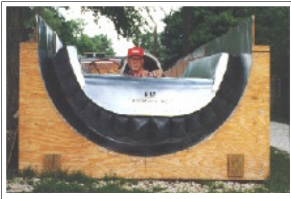
Figure 4. The Aeromobile 17 on cushion at the end of the ROW, with 1 or 2 inches of free air space between the skirt tips and the sheet metal guideway. This renders it totally frictionless, perfectly centered, and positively confined to the groove ROW.
